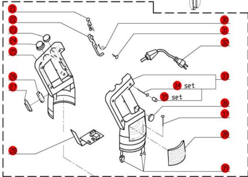
**If replacing internal parts within dashed lines, order a set of replacement screw caps, part # MP29544.**
